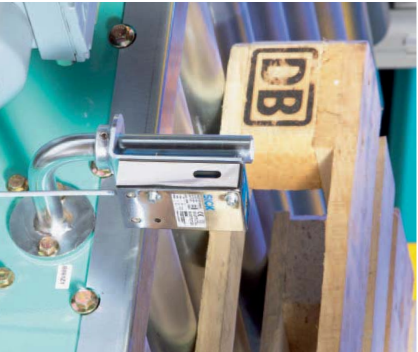
▼ WTB27-3Ex photoelectric proximity switch detects the presence of pallets.
